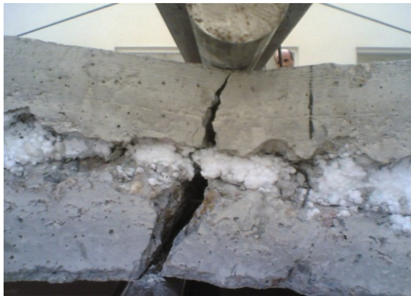
Figure 7: Cracking Pattern for Two-layer Panel in Shear Test
