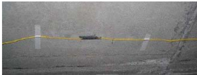
Fig. 8 Surface mounted FBG strain sensors
